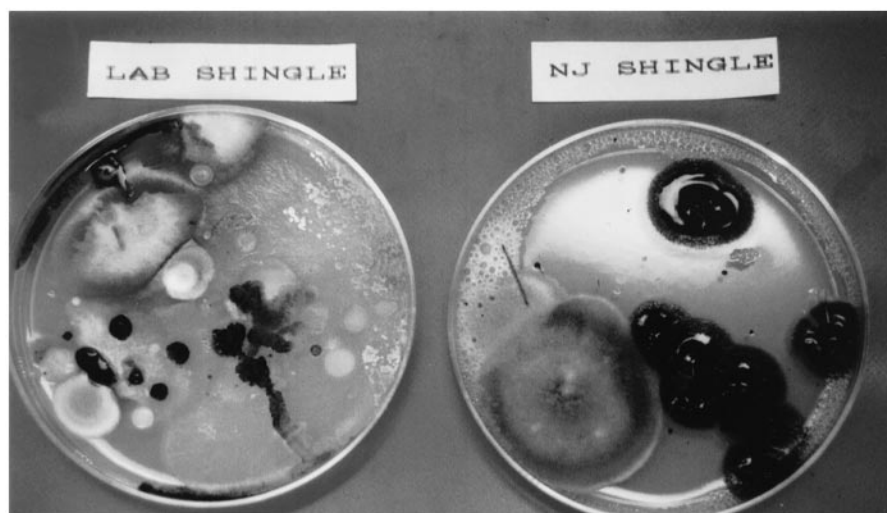
Figure 1 Recovery of fungi from cedar shingles—comparison of isolates from maritime (laboratory) and inland (New Jersey) locations. Cultures were grown on potato dextrose agar. No major distinction was found between the isolates from either location, and Aureobasidium pullulans , the black slimy yeast, was always isolated from both sites.
